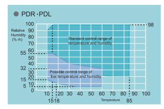
The above performance is measured in the ambient temperature of +  $23\,^\circ\text{C}$ , without any load and heat dissipation.
