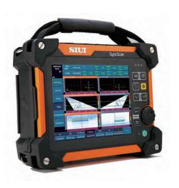
Latest ultrasonic flaw detector from SIUI, SyncScan incorporates the latest advancements in high-performance Phased Array and TOFD detection into one compact and durable unit. SyncScan can be upgraded with Phased Array and TOFD to satisfy various inspection requirements.
